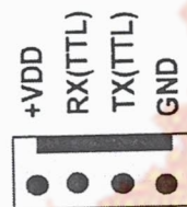
Figure 2.5 displays Connector RS232-TTL(UART) for reading Key Code in the format of ASCII CODE.
