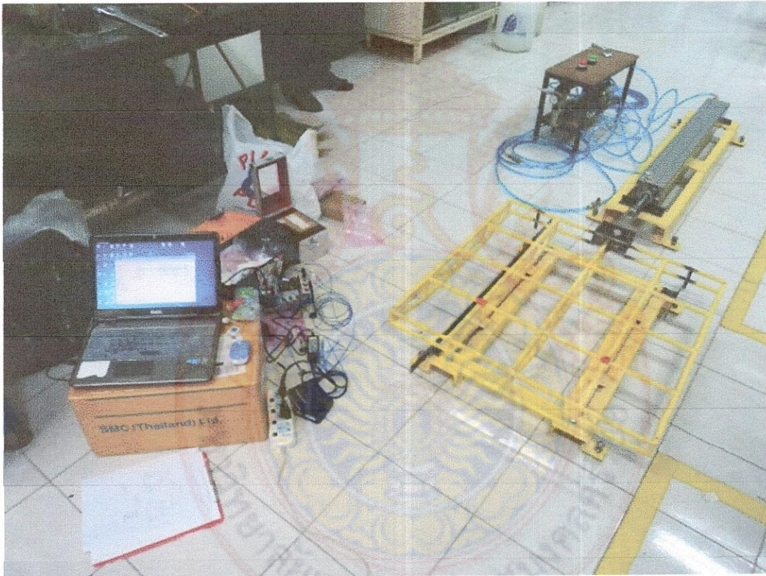
Figure 3. 9 Final assembly of the table attached with accelerometers and data acquisition system readily for shaking test
