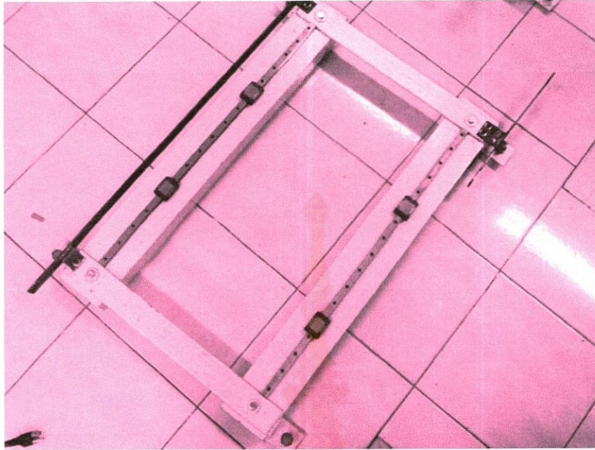
Figure 3. 5 Stainless steel rail guides fixed on a steel platform
